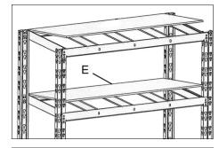
We recommend that the racking be secured to an adjacent wall using typical wall insert plugs and screws (not supplied) aligned with the assembly slots in the posts.
